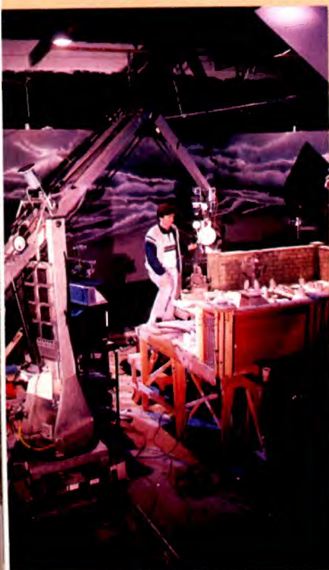
Cinematographer Pete Kozachik, filming a real-world cemetery with the Luxo Sr. motion-control rig.
